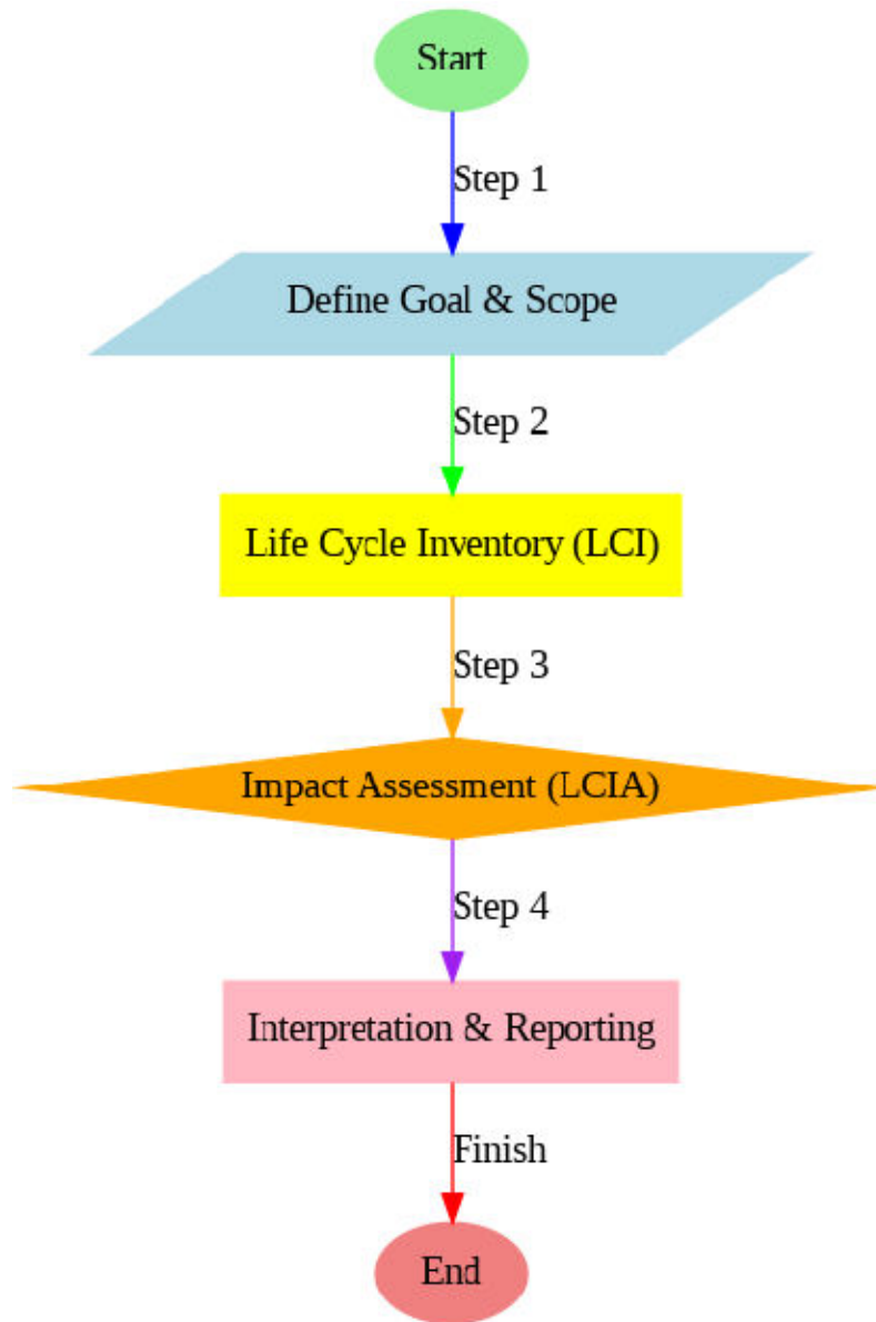
Figure 2: Flowchart of the step-by-step LCA process, illustrating data flows and analysis stages.
